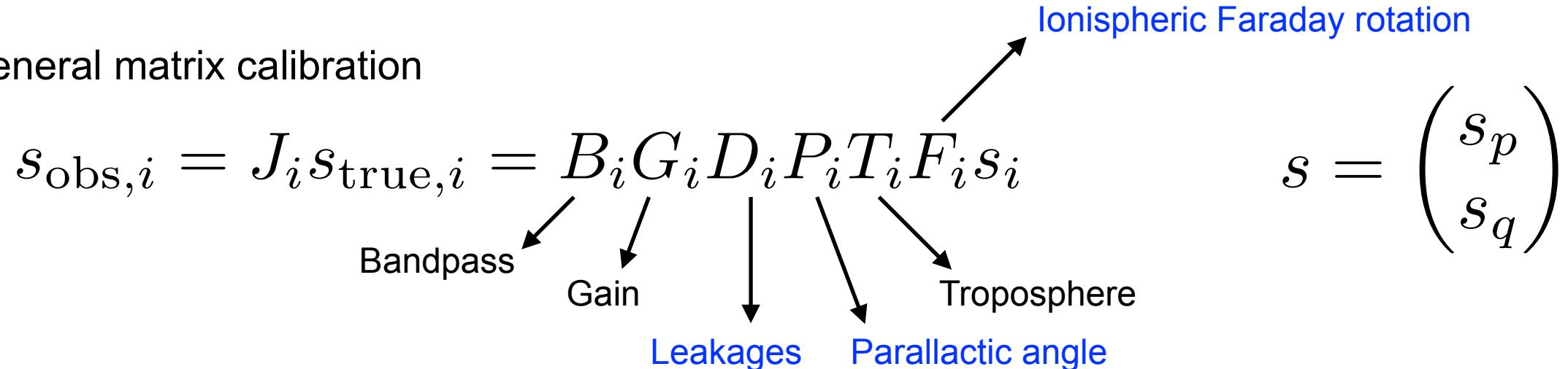
We can imagine each antenna's received signal corrupted from right to left by the different factors
