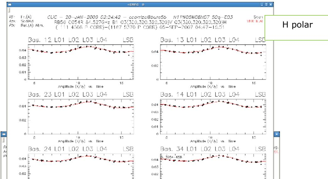
NOEMA H and V amplitudes with a polarized calibrator
